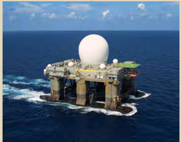
Figure 3 Raytheon built the X-Band Radar (XBR) portion the Sea-Based X-Band Radar (SBX). As a key part of the Ballistic Missile Defense System (BMDS), the XBR can be positioned in the ocean to support both testing and provide radar coverage for possible threat missile launches throughout the world.
